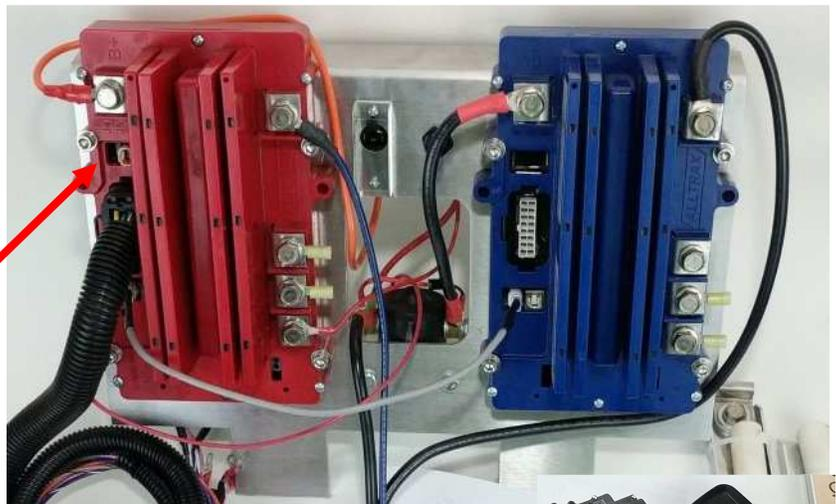
If you have the Alltrax SOC fuel gauge meter plugged into the BMS J5, remove it from the BMS. Then - on the BLUETOOTH MODULE, remove the CAN TERMINATOR PLUG by pressing the TAB, and then plug the SOC Fuel Gauge CAN cable into the RIGHT SIDE connector of the Bluetooth Module.
