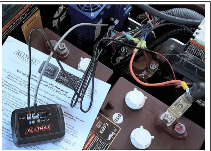
8. Find a location under the seat – fender, or side panel to mount the BLUETOOTH MODULE. Vertical is preferred so water can drain away from the unit.
