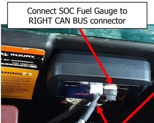
Connect SOC Fuel Gauge to RIGHT CAN BUS connector
